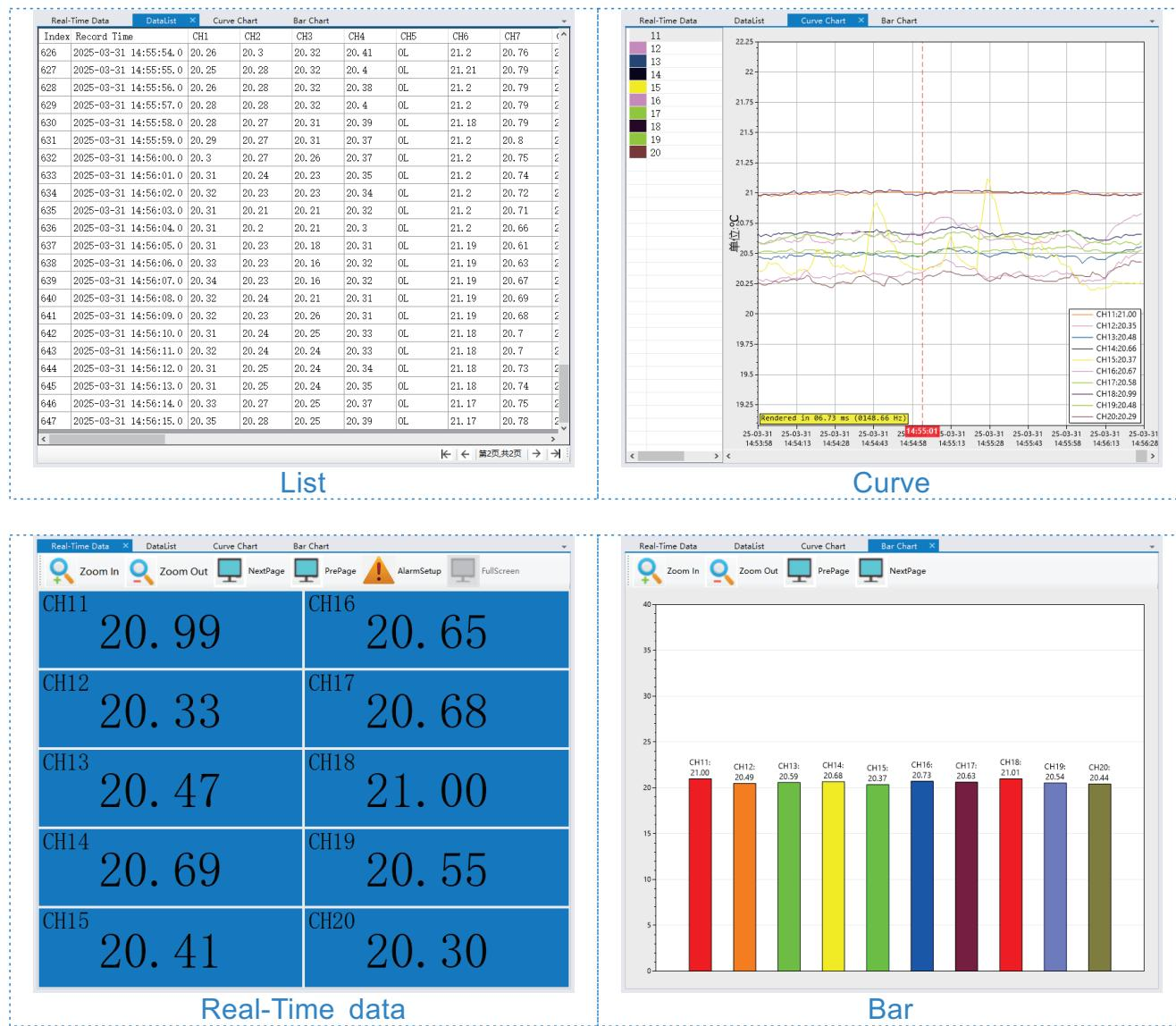
Each data list can move the list position and size as needed. Take the curve list and bar chart list for example, where the curve list is the moving list and the bar chart is the selected list.
