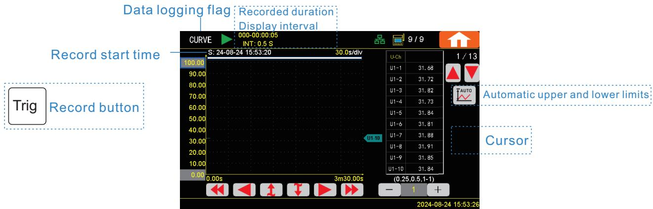
Click on the cursor button to show the cursor in the axes and click again to hide the cursor. Move the cursor with the left/right shift keys. Click on Auto Coordinate to automatically set the upper and lower limits.
