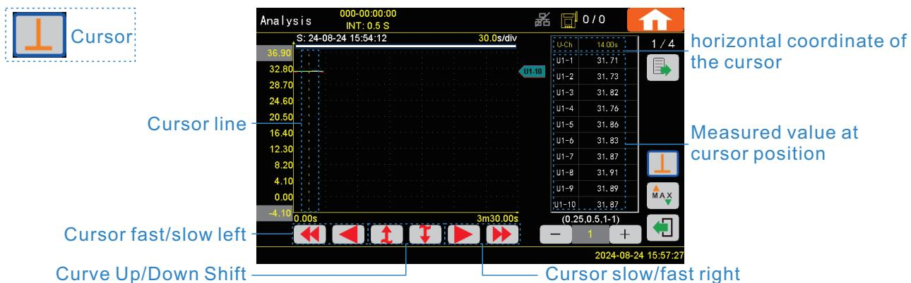
Click the Max/Min button to bring up the selection interface, select the jump value and channel, then press OK to jump.
