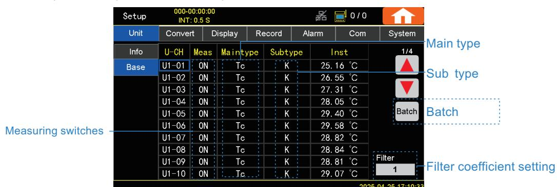
Module channel type settings can be set in batch.
