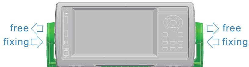
The handle has a total of 5 fixing positions.
