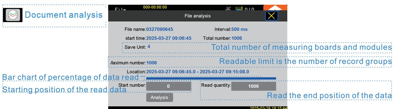
After setting the data interval for analysis, enter the analysis page. In the page, you can click the vertical coordinate upper/lower limit to modify, zoom in/out the curve horizontally, call out the cursor to read the curve value, and quickly jump to the maximum/minimum value.
