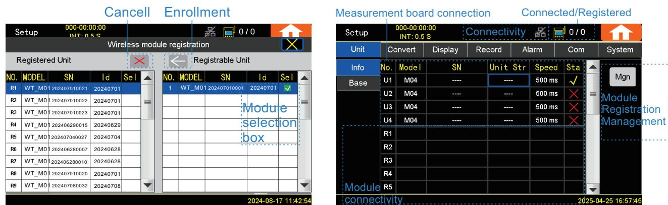
The main interface of the main unit can control the channel switch, switch between primary and secondary types, and set the measurement filter coefficients of the measurement board.
